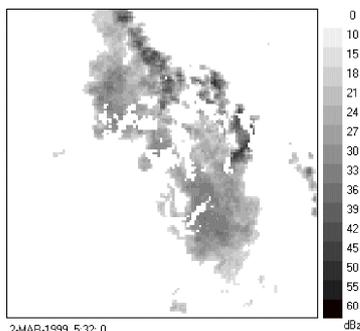
Figure 5.2. Rain field measured by the Melbourne weather radar on 2 March 1999. The domain of the field is 256 km and the spatial resolution is 2 km.
