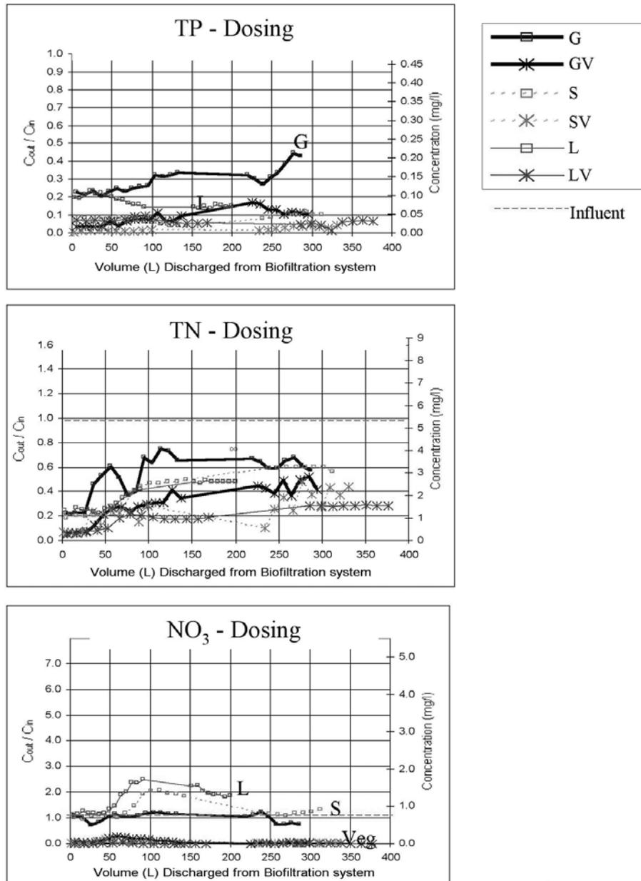
Figure 4.2. Concentration of nutrients in biofilter effluent - dosing experiment
