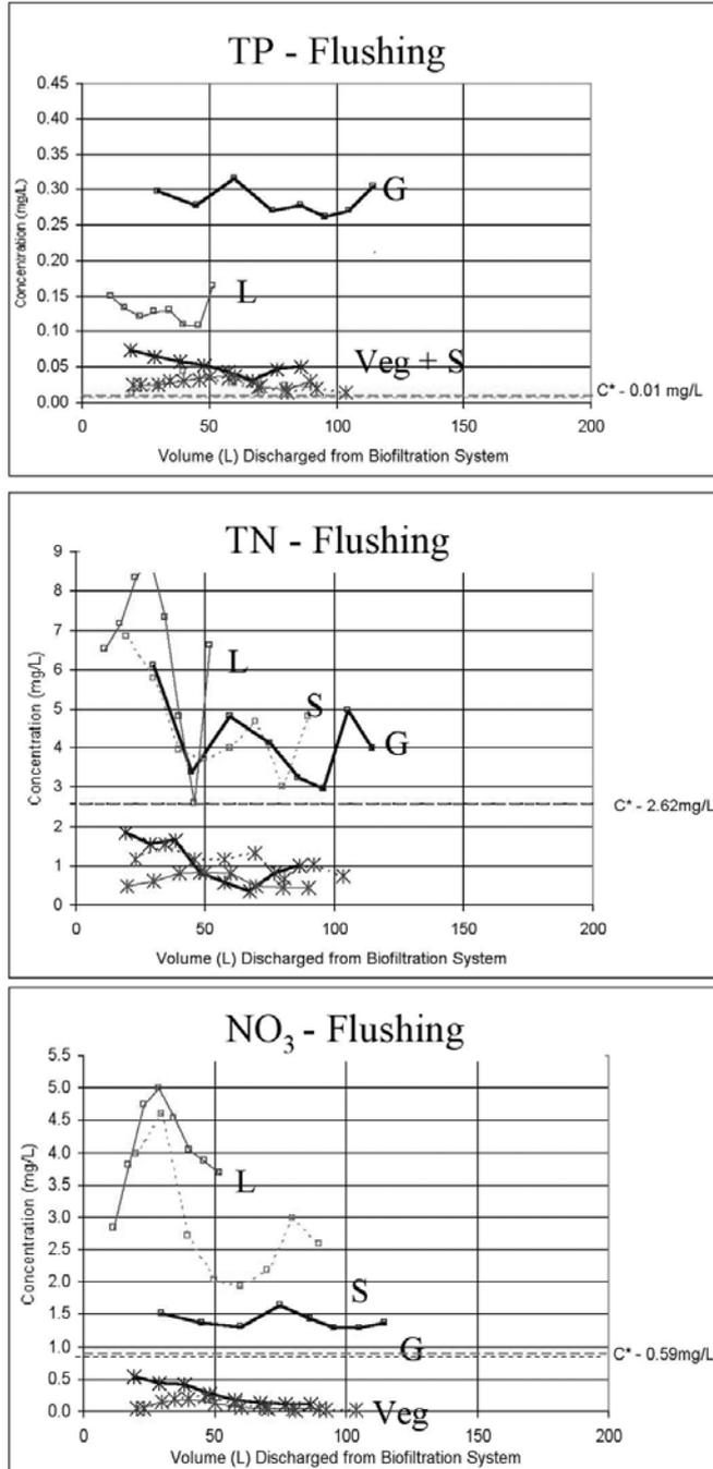
Figure 4.3. Concentration of nutrients in biofilter effluent - flushing experiment
