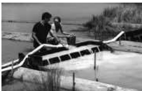
Figure 2 Dosing Sediment Tracer into the Control Channel
