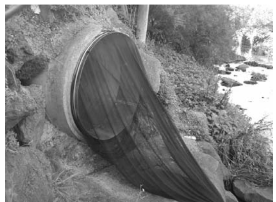
Figure 4.1. End-of-pipe net for downstream monitoring of GPT performance.
