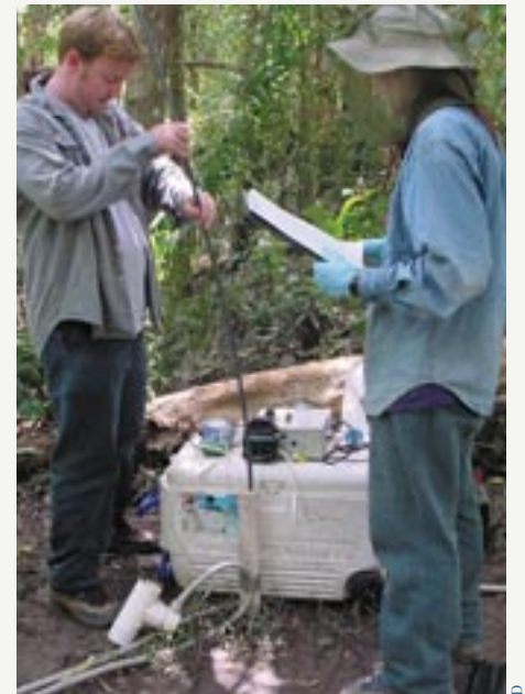
Figure 7. The push–pull technique, where solutes (nitrate, acetate and a tracer) are pushed a short distance from a well into the perched water table and then pumped out again some hours later. The ratio of nitrate and tracer in the recovered solution is then compared with that in the solution pumped into the well, to estimate the amount of nitrate removed.
